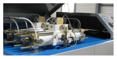
As the only French manufacturer of ultra high pressure amplifiers and pumps, HYDROPROCESS develops specialised machines for a wide range of applications, including industrial waterjet cutting machines (food processing and manufacturing) and for explosive device neutralisation systems (civil and military security), ultra-high pressure amplifiers
